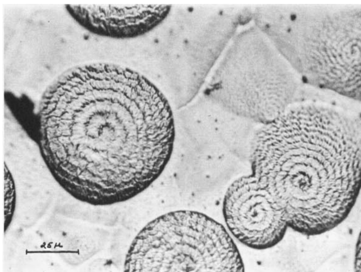
FIG. 4. Banded spherulite of polyoxymethylene prepared by evaporation at room temperature of a hexafluoroacetone sesquihydrate solution. [O'Leary, (19).]
