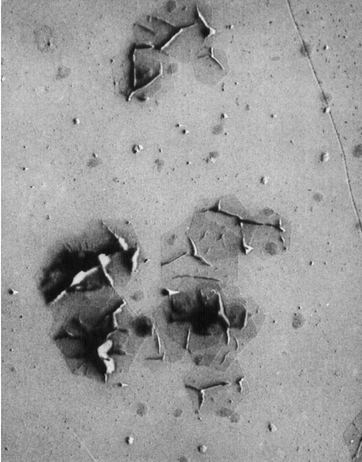
FIG. 1. Polyoxymethylene crystals grown from a 0.05% solution in bromobenzene at 115°C. (Micrograph of C. A. Garber.)
